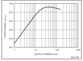
Figure 17. Output noise versus output current.
