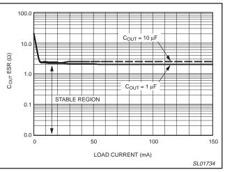
Figure 14. Region of stable C<sub>OUT</sub> ESR versus load current.
