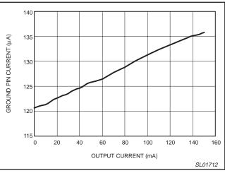
Figure 4. GND pin current versus output current.
