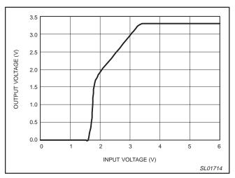
Figure 6. Output voltage (I<sub>OUT</sub> = 50 mA) versus input voltage.
