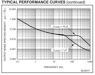
Figure 13. Output noise spectral density versus frequency.
