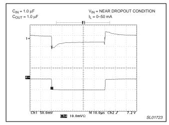
Figure 20. Load transient response.
