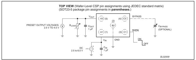
Figure 1. Simplified system diagram.
