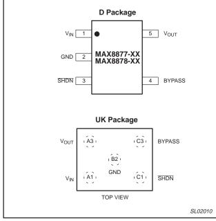
Figure 2. Pin configurations.
