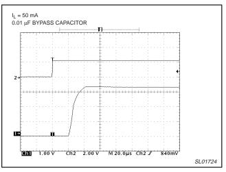
Figure 21. Shutdown exit delay.
