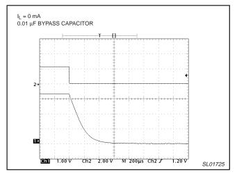
Figure 22. Entering shutdown (no load).
