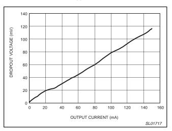
Figure 8. Dropout voltage versus output current.
