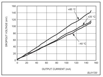
Figure 12. Dropout voltage versus output current.
