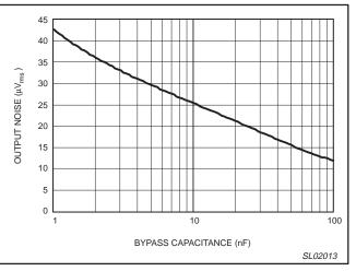
Figure 16. Output noise versus BYPASS capacitance
