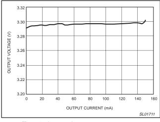
Figure 3. Output voltage versus output current.
