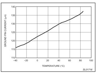
Figure 10. GND pin current (50 mA load) versus temperature.
